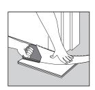
If a door frame needs to be cut, use a piece of plank to obtain the correct height.
